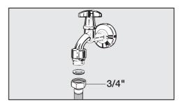
Screw the supplied brass compression fitting, with the 3/4" end, tightly onto the water connector of the coffee machine. (Tighten the compression fitting by hand, do not use a tool.) The fitting includes an opening for standard 1/4" piping.
