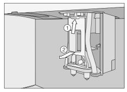
Press the catch upwards ①, grasp the dispensing unit by the handle, and pull it forwards and off ②.
