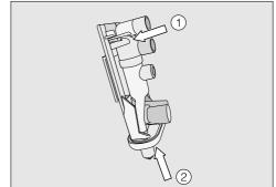
Reassemble the dispensing unit in the reverse order. Make sure that upper adapter ① clicks into position.
