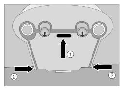
To remove, press and hold the sensor cover between the dispenser nozzles
